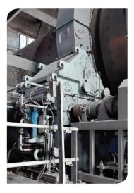
confirm that we have not had to perform an oil change or service the gearbox internals. This is indeed a maintenance-free solution that very clearly saves us money." Afifi further notes that the company does not have to pay extreme attention to the sealing of the rim guard either.
