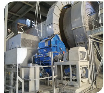
Above: A Lateral Gear Drive designed and manufactured by Wikov drives a horizontal ball mill at a cement plant in North Africa.
