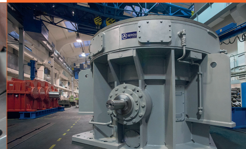
Vertical mill gearbox after refurbishment and upgrade
