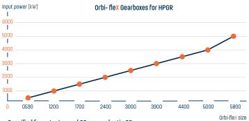
Specified for output speed 20 rpm and ratio 80
