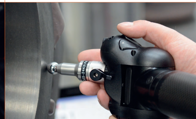
Mobile 3-D measurement of gearbox dimensions
