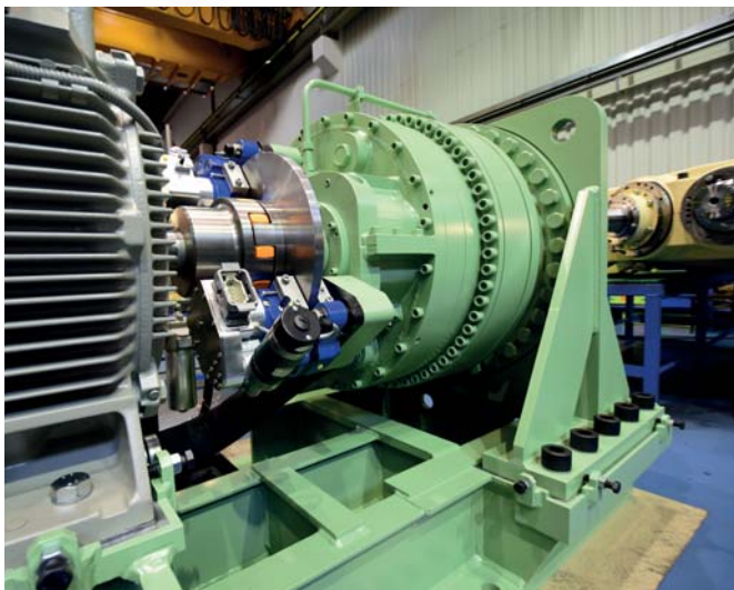
Two-roll mill drive with Orbi-flex® gearbox
