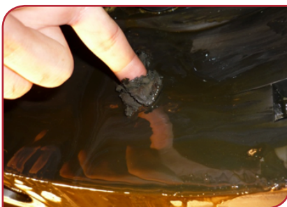
Below: Common oil contamination on conventional side drive solutions that lead to fatal damage of bearings and scoring of gear teeth.
