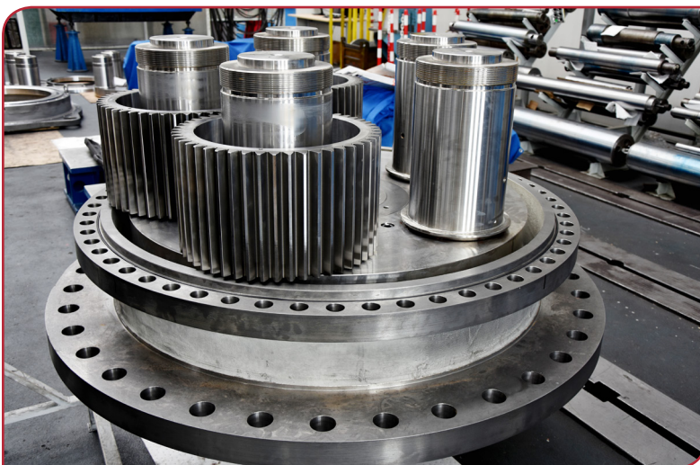
Below - Figure 1: Multi-satellite planetary stage of the Wikov Orbi-flex gearbox during assembly.
