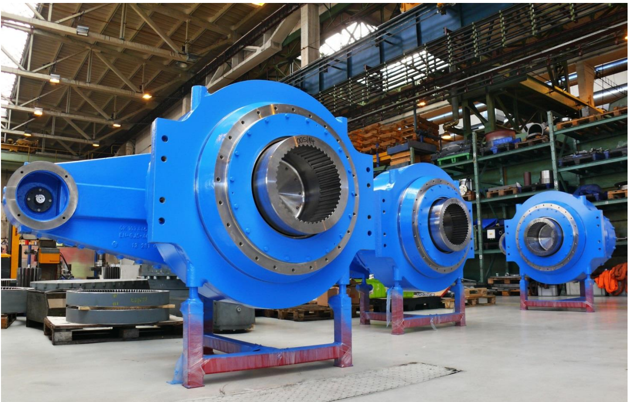
Jacking gearbox for GustoMSC
